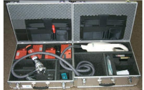
Put the ready-to-use drilling machine with the connected vacuum cleaner on the ground to be drilled. Make sure that the three support feet of the protecting cap are standing safely and firmly.
