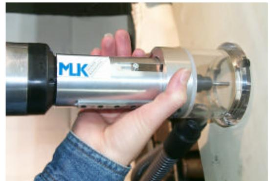
The drill may not touch the ground to be drilled when standing still. Set the drilling machine with the rotating drill vertically on the underground to be drilled. Drilling shall be carried out at intervals and not in one go. Press the drill manually about 1 [mm] deep into the material. Having done this, remove it from the drilled hole to remove the dust from the diamond coating. Read the realized drilling depth from the trailing ruler on the drilling machine.
